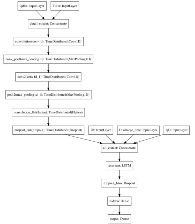
Fig. 4. Full-structure interpretation of the CNN-LSTM model: The Convolution layer handled Qdlin and Tdlin and concatenated with IR, discharge time and QD followed by LSTM.
